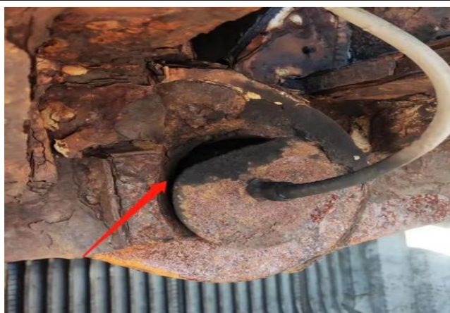
Intermediate hinge was worn out heavily
