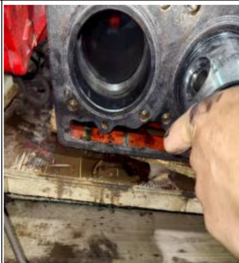
Check the piston and measure the clearance.
