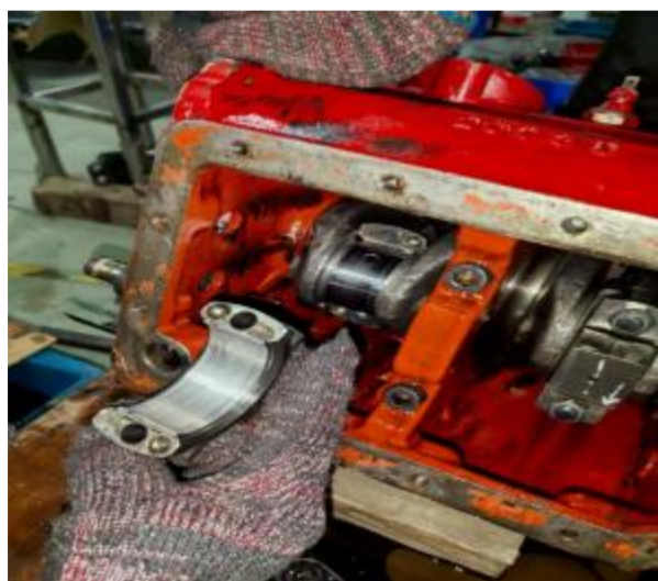
The connecting rod and crankshaft have abrasion.
