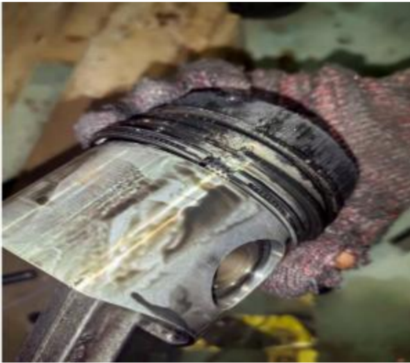
The piston ring clearance is excessive and no tension.
