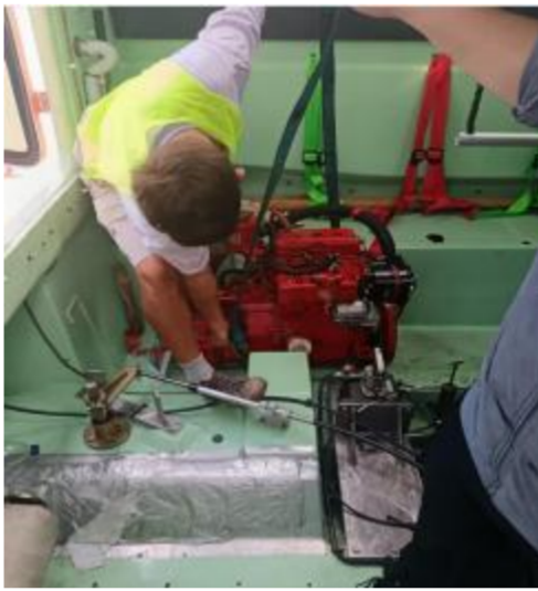
Lift out the engine and offland.
