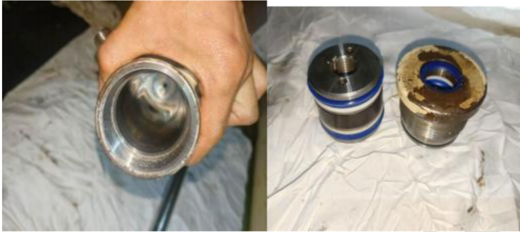
Port side valve block overhauling/Pressure gauge renew.
