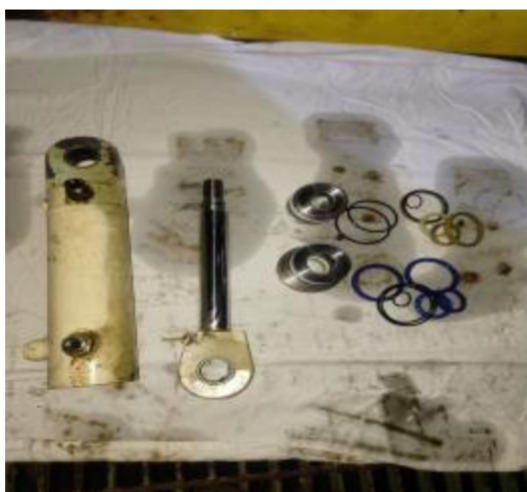
Cleat cylinder overhauling :
