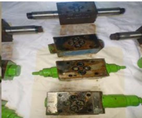
Valve block overhauling and pressure gauge renew.
