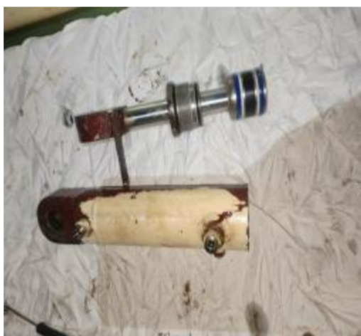
Port side cleat hyd cylinder overhauling :
