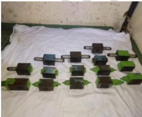
Valve block overhauling and pressure gauge renew.
