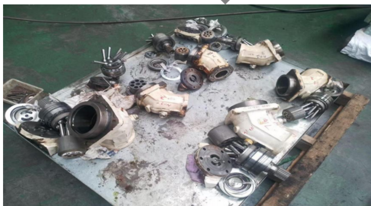
Overhaul the luffing motors in workshop
