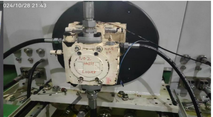
Hoisting pump test by test bench
