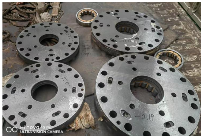
Side covers after repaired
