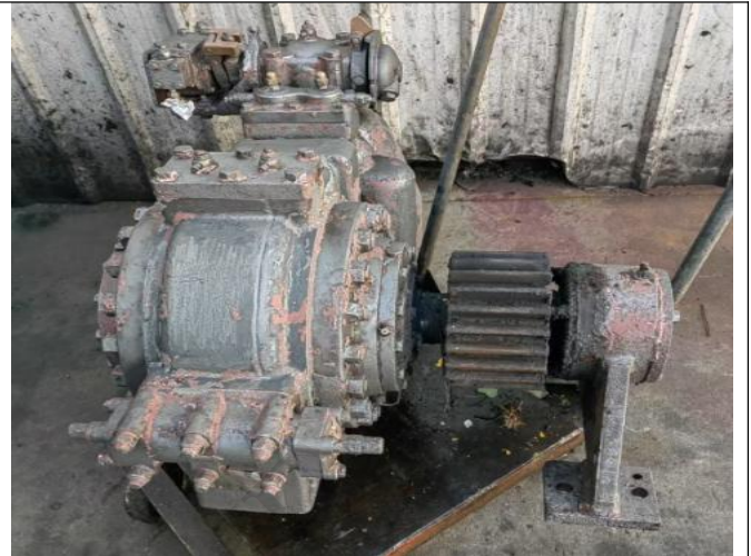
After sand blasting
