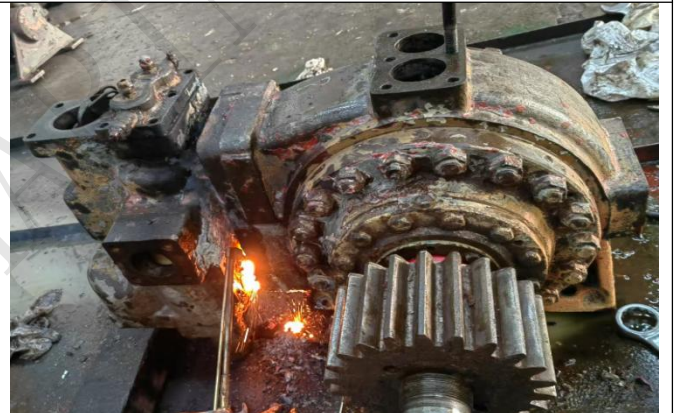
Disassemble the hydraulic motors
